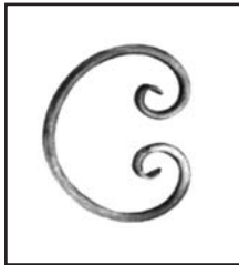
STEEL SCROLL 9/16" round. 6 1/2" wide x 8 7/8" high. Weight 1.6 lbs. AMC6348
