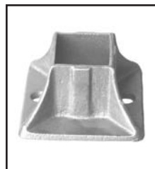
CAST IRON SHOE 3 3/4" x 3 3/4". 2" deep collar. Fits 1 1/2" square tube. FECCEHH
